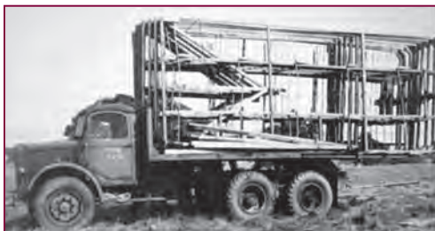
Fig 2. The portable broadside array used by Das Gupta in 1951 [Ref-4]
